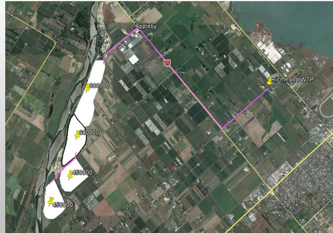
4 storage ponds along the river to allow for 2,300,000m 3 storage, piped to Richmond water treatment plant in underground pipes along existing arterials.
