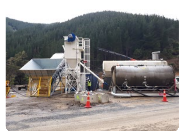
Onsite concrete batching plant built in 2019.
